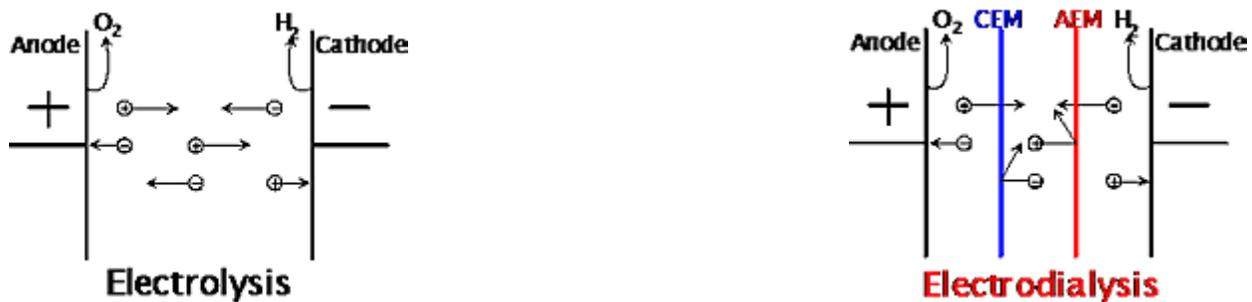
**Figure 1. Left side demonstrates a standard electrolysis process. Right side demonstrates the same process when ion-selective membranes are inserted.**
